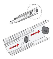
The rubber stops of type F dampen the impact of the slide in the respective end position. This feature minimizes noise development and increases the lifespan. Attached to the slides in a partially concealed, partially visible manner, the stops meet each of the requirements in regard to shape, material, and hardness.
