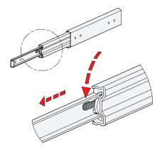
Type F has additionally a detach function through which the extension slides can be completely separated from one another in the area of the middle and inner slide. This feature not only facilitates mounting. It also allows the extension to be quickly removed, for example, when frequent maintenance work is performed on the components located behind.
